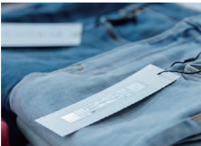
RFID tags can be read from any directions, unlike barcode tags.
